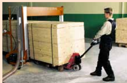
Between the cuts you move the package with a standard pallet jack.
